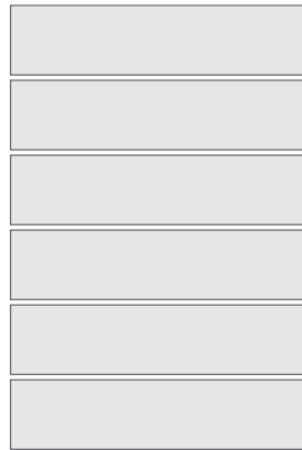
单粒 Chipsize: 45X195mm (2"X8") 联长 Sheetsize: 291X198.5mm 灰缝 Joint Width: 3.5mm
